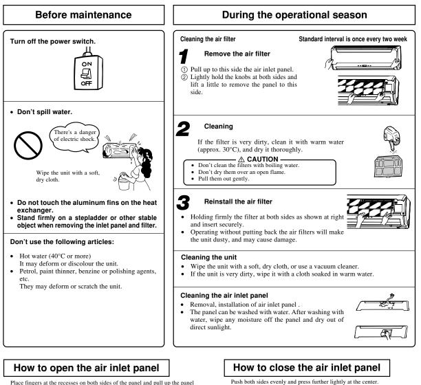
Place fingers at the recesses on both sides of the panel and pull up the panel to this side so that it will be opened by about 60 degrees.
