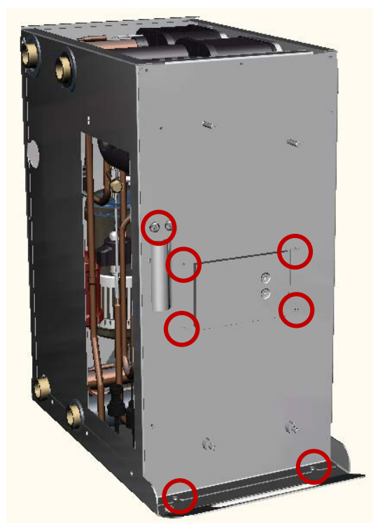
Step 16. Dismount plate to refrigerant circuit, 4 screws (Torx T20) and 2 screws (Torx T30) for staple and 2 M6 nuts.
