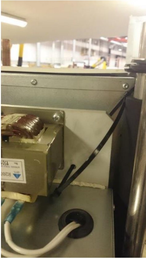
Step 11. Detach inverter in upper edge. Install 2 cable ties in series.
