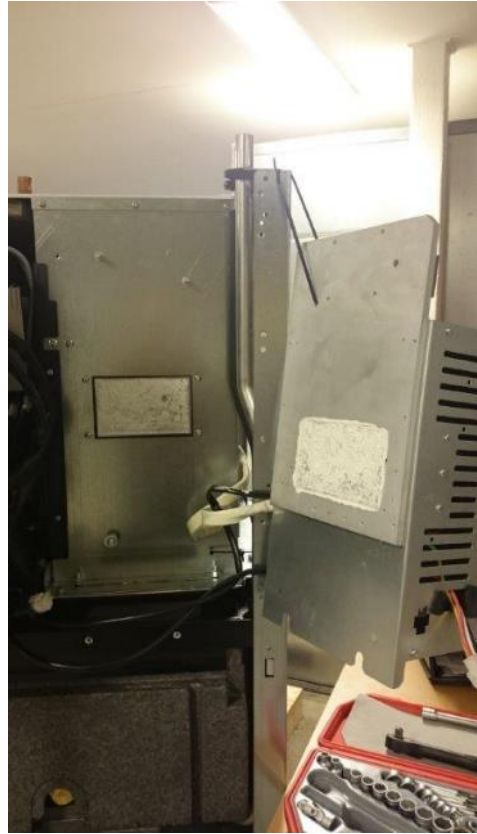
Step 12. Hang inverter on the right pillar/corner profile.
