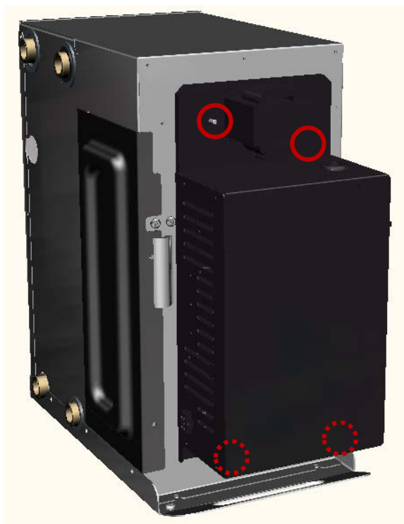
Step 14. Dismount inverter, 4 nuts M6 (socket No 10).
