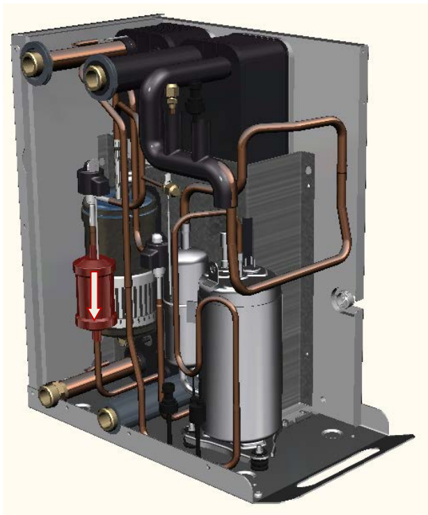
Step 24. Mount compressor. Solder the filter dryer and compressor. Note! Use nitrogen as protection gas and cool exp.valve with wet cloth. See filter flow direction.
