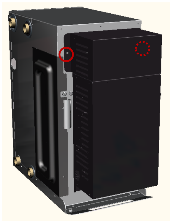
Step 13. Remove lid for DC choke coil (Torx T20).
