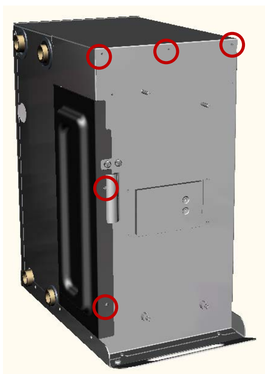
Step 15. Dismount top and service hatch to refrigerant circuit (Torx T20).
