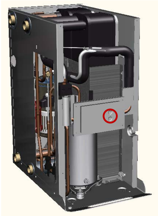
Step 17. Dismount cooling plate for inverter (Torx T20).
