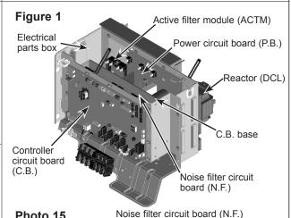
Photo 15 Noise filter circuit board (N.F.)
