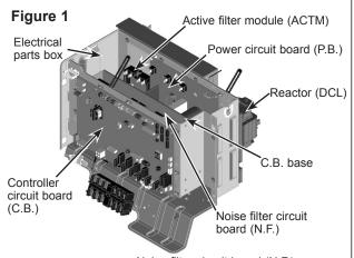
Photo 15 Noise filter circuit board (N.F.)
