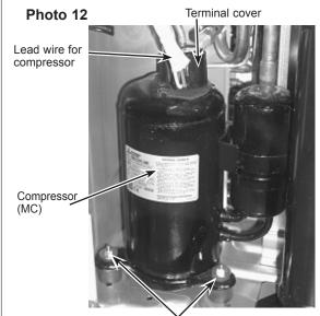
Compressor fixing nuts
