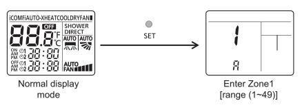
To enter zone 2 area: (Press set continuously for T ≥ 5 secs)
