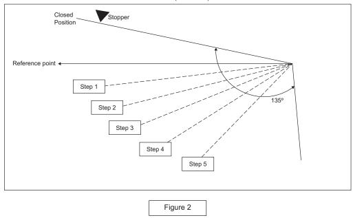
\* The horizontal vane angle tolerance is within +/- 5 degree.
