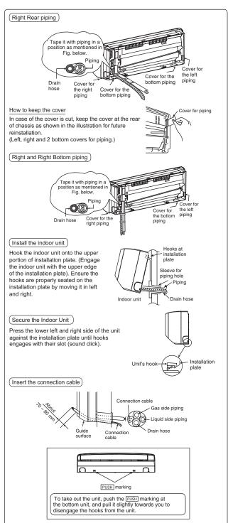
(This can be used for left rear piping and left bottom piping also.)
