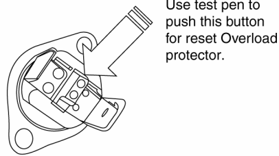
How to reset Overload protector
