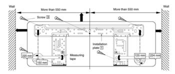
The centre of installation plate should be at more than 680 mm at right and 570 mm at left of the wall.
