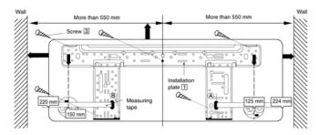
The centre of installation plate should be at more than 550 mm at right and left of the wall.
