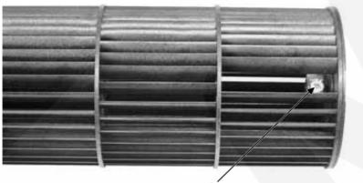
2 Remove the screw that holding the cross flow fan and fan motor axis.
