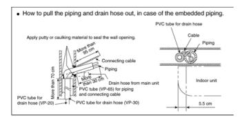
• In case of left piping how to insert the connecting cable and drain hose.
