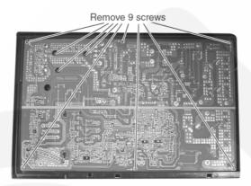
▲ Caution! When handling electronic controller, be careful of electrostatic discharge.
