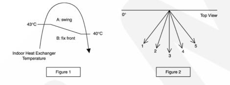
2. Manual horizontal airflow direction can be set using remote control; the angles of the vane are as stated below and the positions of the vane are as Figure 2 above.
