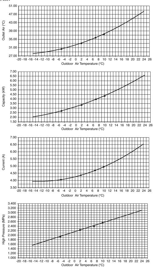
[Condition] Indoor temperature: 20/-°C, 7/6°C Remote condition: High fan speed, Heat 30°C
