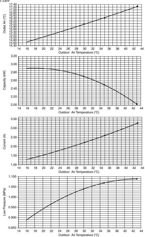
[Condition] Indoor temperature: 27/19°C, 35/-°C Remote condition: High fan speed, Cool 16°C
