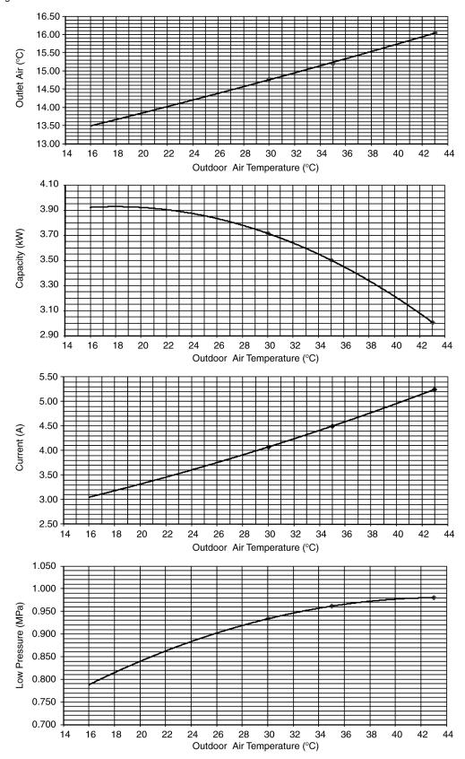
[Condition] Indoor temperature: 27/19°C, 35/-°C Remote condition: High fan speed, Cool 16°C Comp. Hz: Rated F<sub>c</sub>
