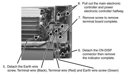
Detach 3 connectors as labeled from the electronic controller. Then pull out main controller gently.
