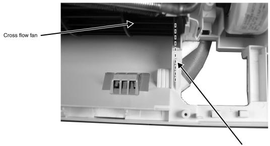
Reminder: To reinstall the cross flow fan, ensure cross flow fan is in line as shown in figure 11.
