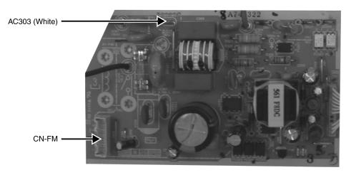
Detach the AC303 and CN-FM connectors from the electronic controller. Then, pull out power electronic controller gently.
