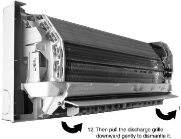
11. Pull out to remove the drain hose from the discharge grille.
