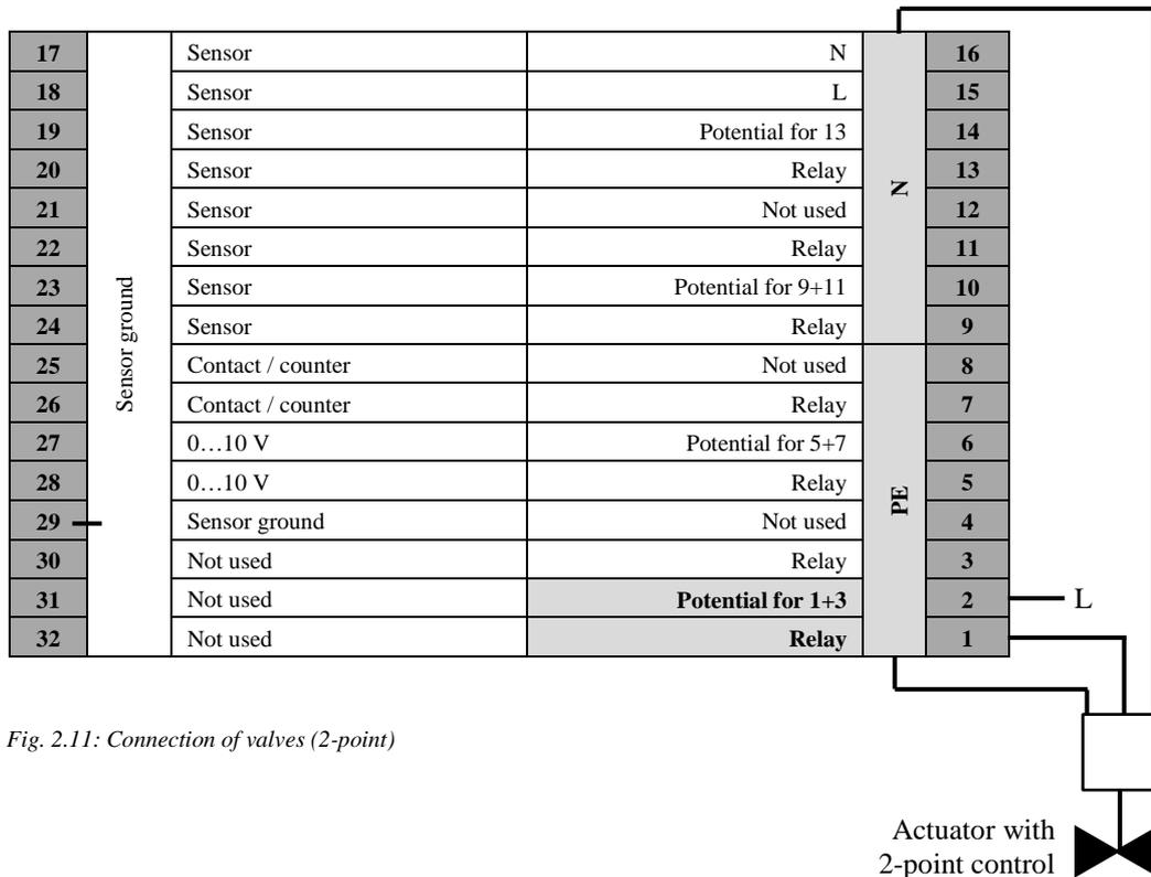
Fig. 2.11: Connection of valves (2-point)
