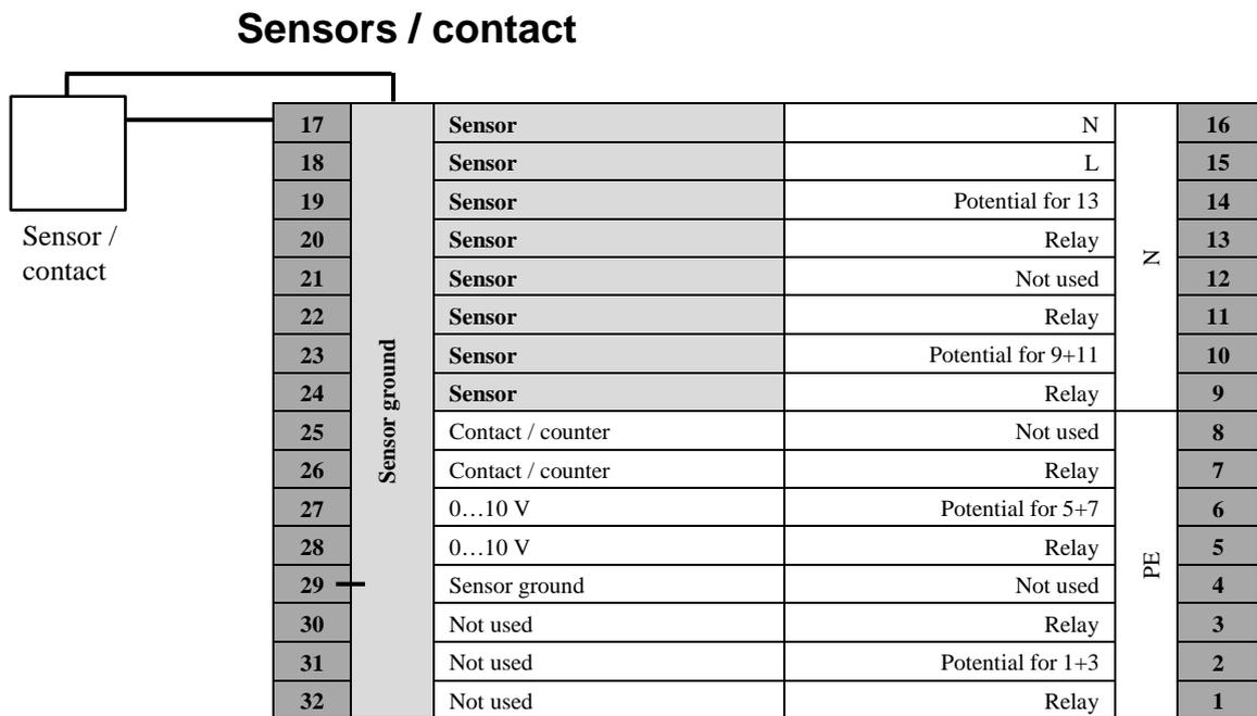
Fig. 2.6: Connection of sensors or contact inputs
