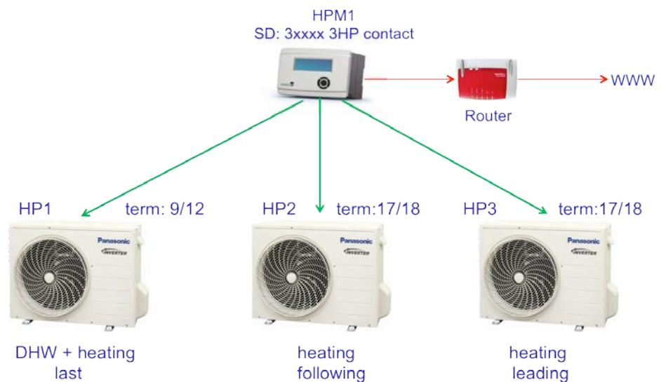
Fig. 2.19: A cascade system using release via contact
