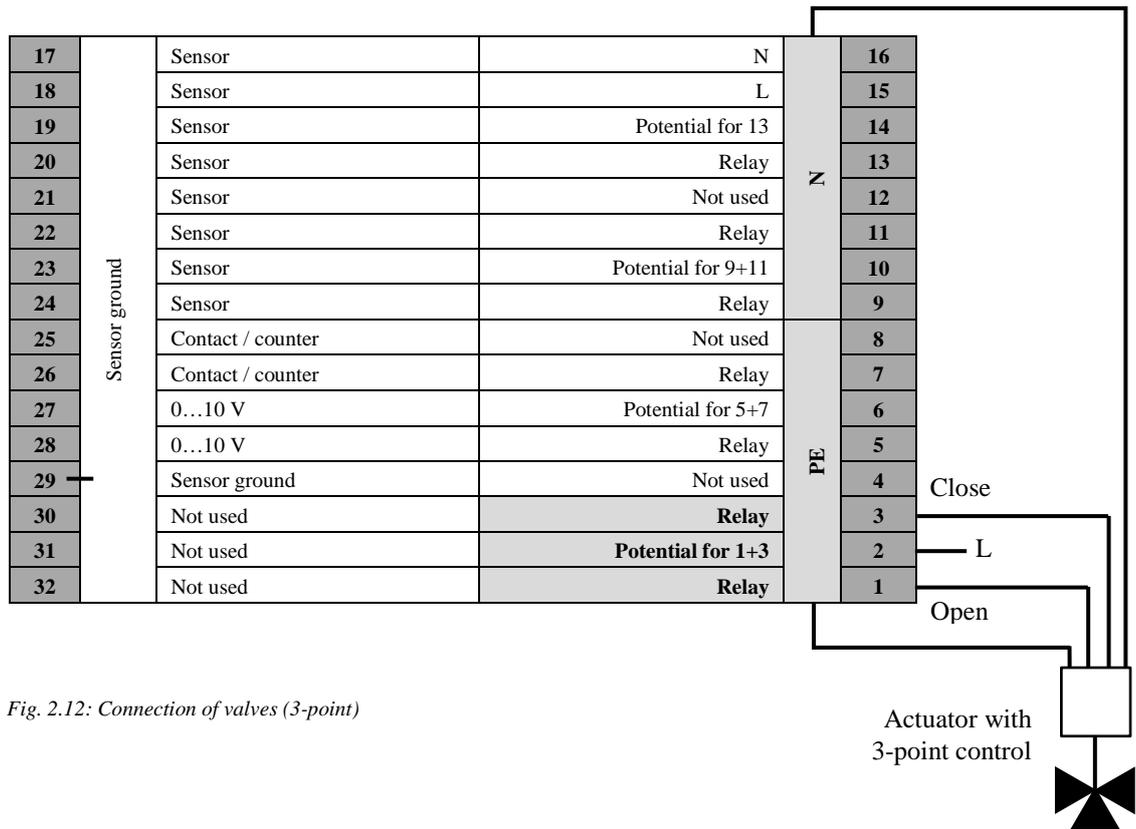
Fig. 2.12: Connection of valves (3-point)
