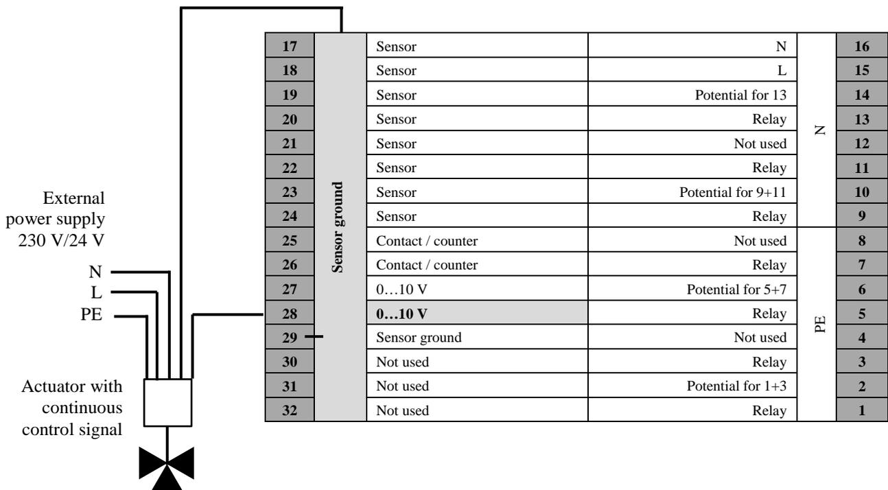
Fig. 2.13: Connection of valves with continuous control (0...10 V)
