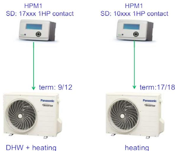
Fig. 2.17: Heat pump activation via contact
