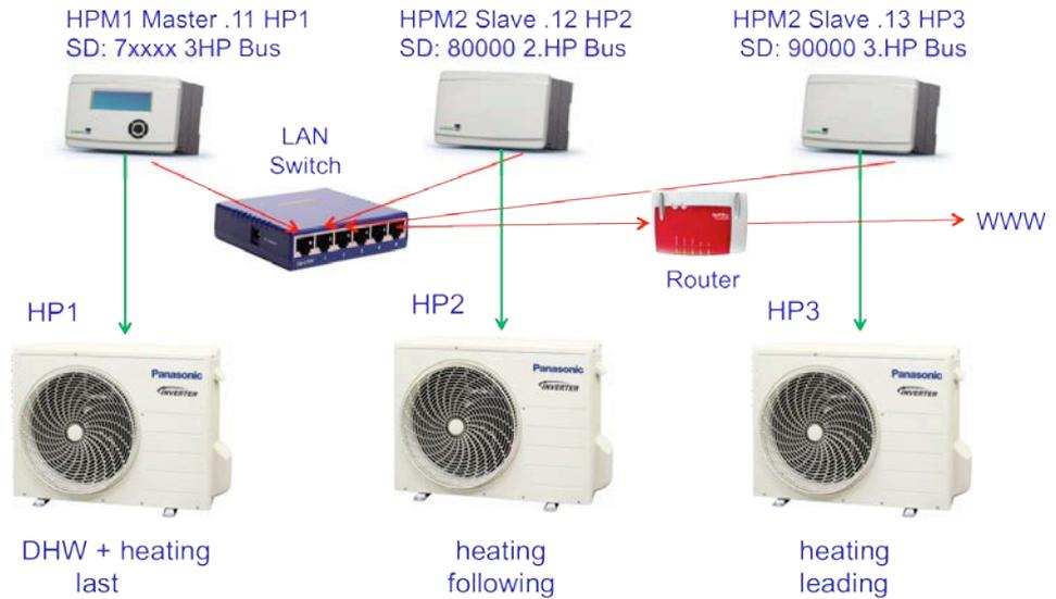
Fig. 2.20: cascade system with communication via BUS
