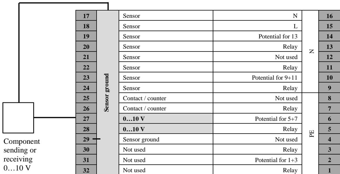
Fig. 2.9: Connection of 0..10V inputs or outputs
