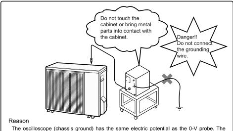
The oscilloscope (chassis ground) has the same electric potential as the 0-V probe. The entire electronic control section of the outdoor unit has a voltage potential difference from the ground as shown in the above diagram. When the oscilloscope is set up, the 0-V line and the ground voltage (ground) will be short-circuited, resulting in an excessive current flow to cause damage to the oscilloscope or indoor electric circuits.
