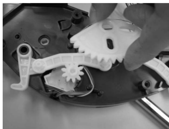
22)The gear, the crank, and the arm are removed.
