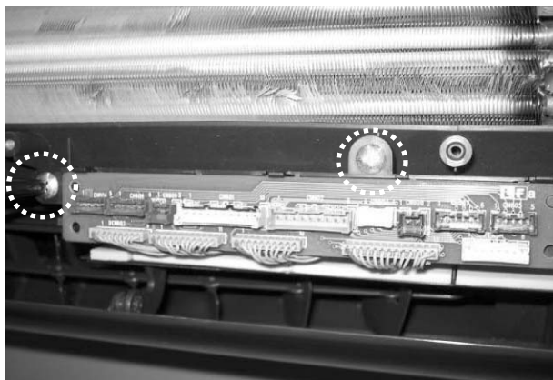
50)P.W.B. assmbly is removed. (2 screws)
