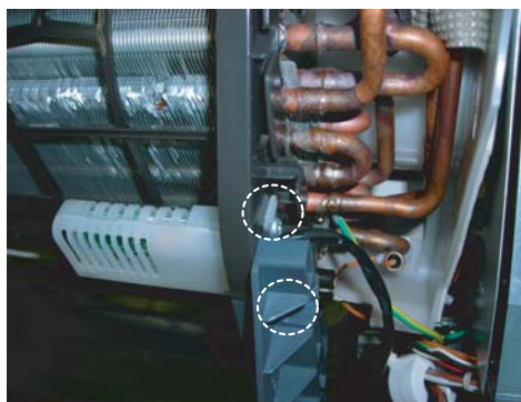
49)The relay printed board holder removed. (2 screws)
