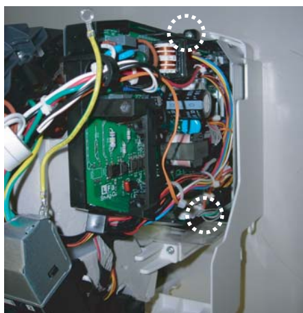
50)P.W.B. assmbly is removed. (2 screws)
