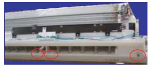
23)Remove the drain pan retaining screws (3).
