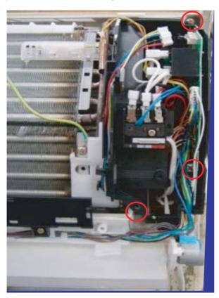
17)Disconnect the connectors ([fan motor / cluster / louver motor] x 2, rimit switch).
