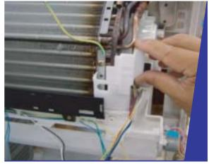
21)Remove the side panel L and drain pan retaining screws (3).
