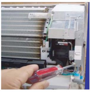
12)Remove the light receiving unit retaining screw (1).
