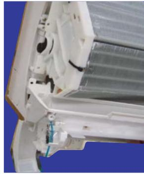
29)Remove the heat exchanger retaining screws (2).
