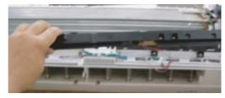
16)Remove the control box retaining screw.
