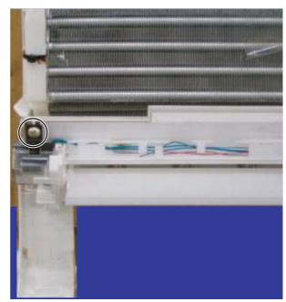
13)Open the 6 tabs on the lead wire guide.
