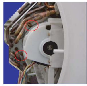
30)Disengage the heat exchanger.
