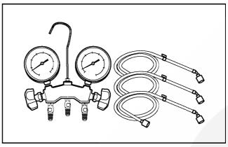
Fig. 4 Manifold gauge charging hose
