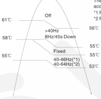
The frequency for the compressor will change according to the outdoor piping temperature. \*1 PE9CKE \*2 PE12CKE
