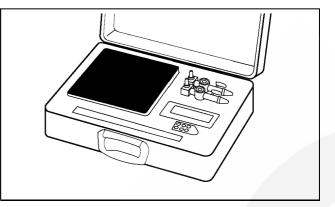
Fig. 7 Electronic scale for refrigerant charging
