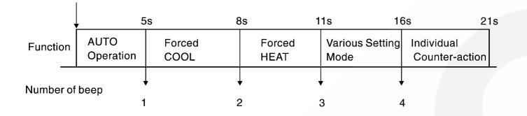
1. When the switch is pressed between 0 to 5 seconds, Auto Mode operation starts to function.
