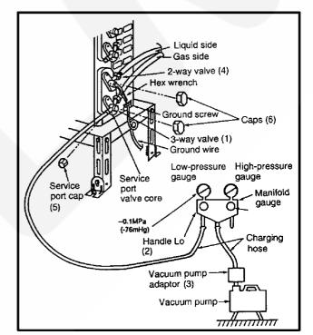
Fig. 12 Vacuum pump air purging configuration
