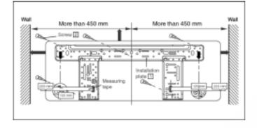
The centre of installation plate should be at more than 450 mm at right and left of the wall.
