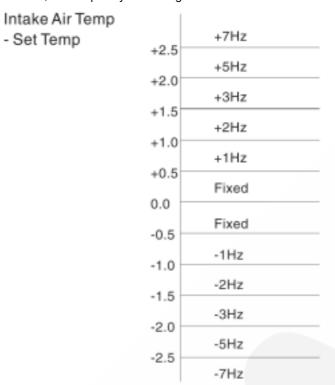
Maximum and Minimum Frequency For Heating Operation
