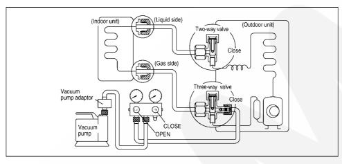
1. Connect a charging hose with a push pin to the Low side of a charging set and the service port of the 3-way valve.
