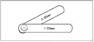
Fig. 1 Copper tube gauge for clearance adjustment
