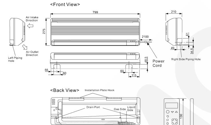
Relative position between the unit and the installation plate<Front View>
