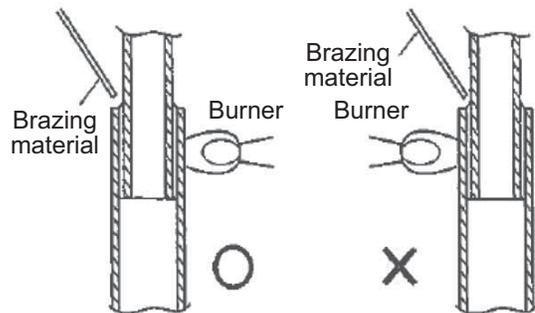
The pre-heating is to heat the base material until the melting temperature, and requires certain training to distinguish the color of the heated base material in order not to melt the material.
