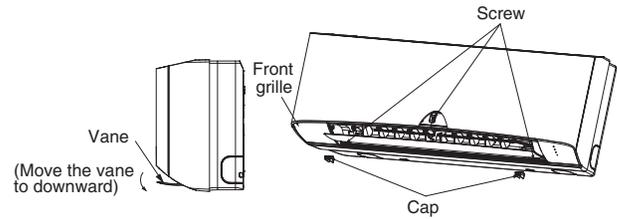
When reinstalling the front grille, carry out above step 2 - 3 in the reverse order.
