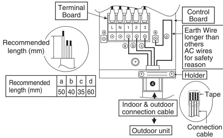
6 Secure the connection cable onto the control board with the holder.
