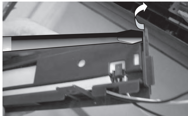
36)Two hooks of the plasmacluster cover are removed by using (-) screwdriver.
