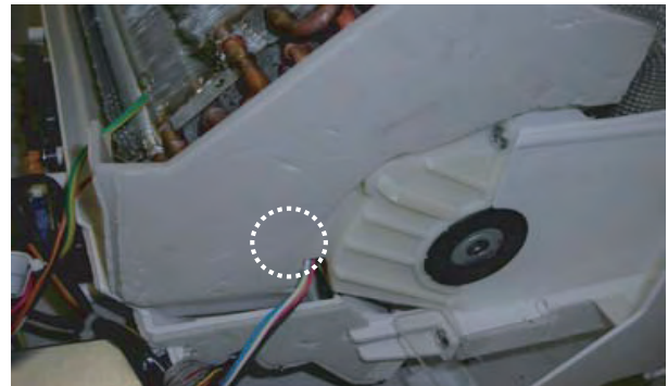
54)The drain pan is detached.
