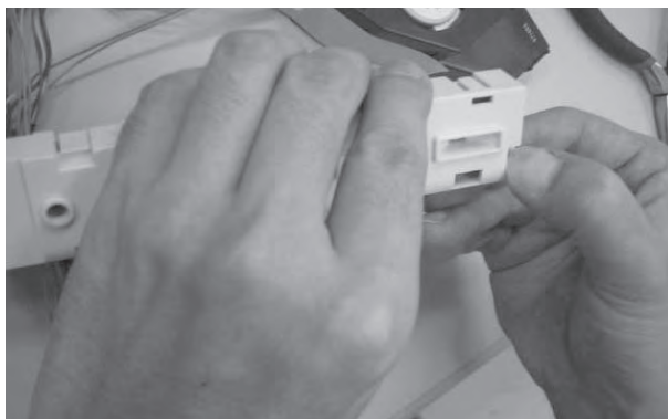
17)The cover of the display printed board is removed.
