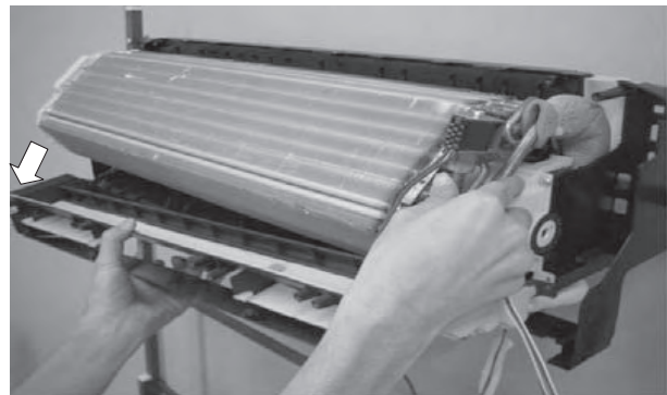
54)The drain pan is detached.
