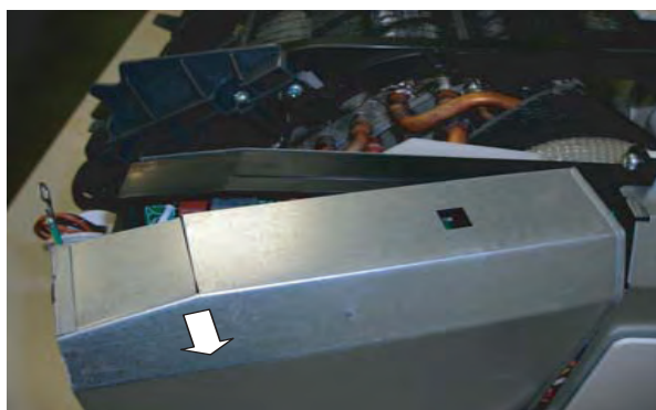
30)The P.W.B. box cover is removed.
