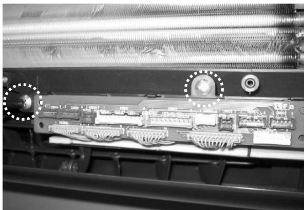
50)P.W.B. assmby is removed. (2 screws)
