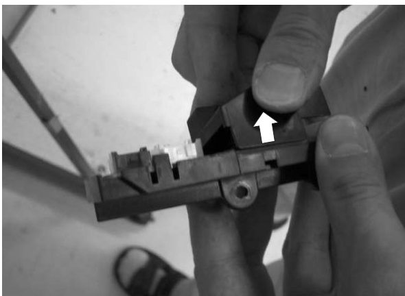
32)The sub.printed board is removed. (Hook two places)
