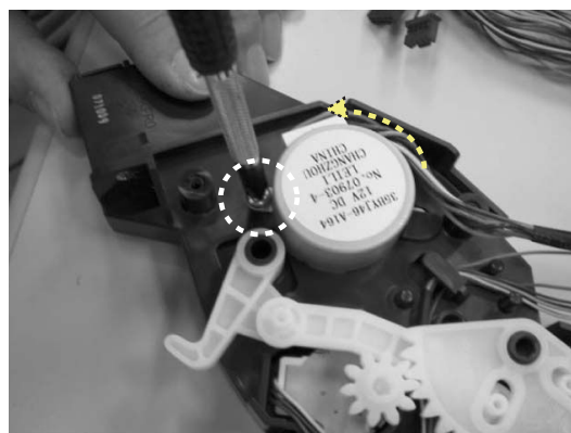
22)The gear, the crank, and the arm are removed.
