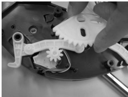
22)The gear, the crank, and the arm are removed.
