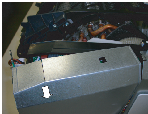
36)The fixing band in the P.W.B. assembly is cut. (4 parts)
