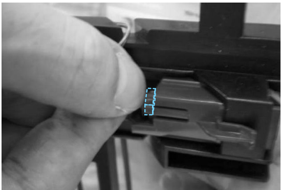
48)The thermally sensitive resistor holder is removed. (Hook two places)
