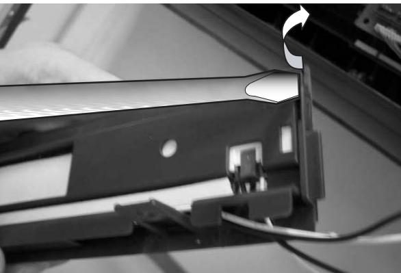
42)After the plasmacluster that removes the PC cover is taken out, the wire connector is removed.
