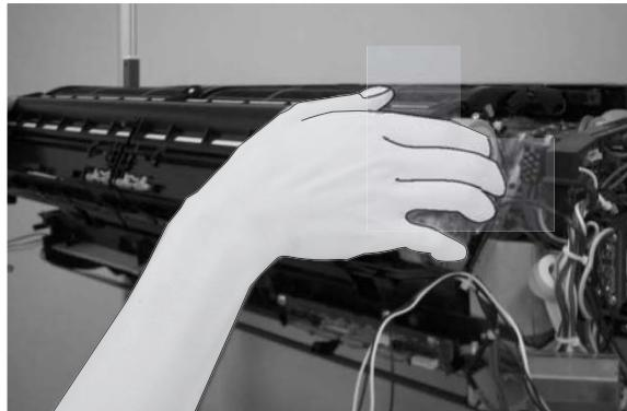
45)The limit switch cover is removed.
