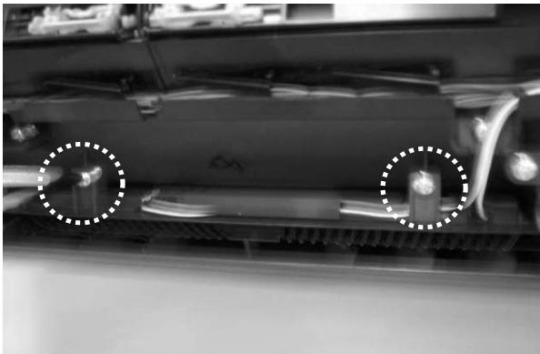
40)The plasmacluster assembly is pulled forward, and detached.
