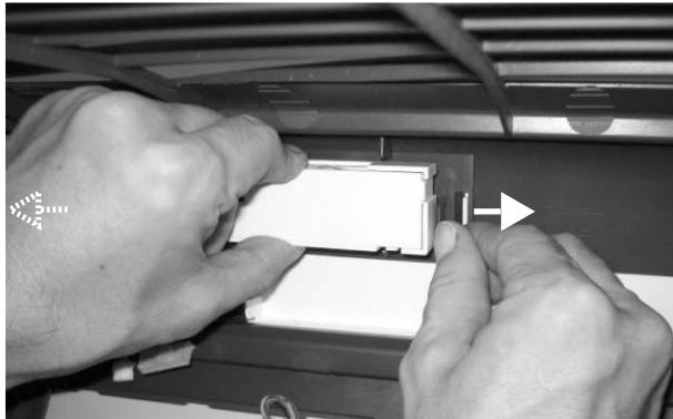
17)The cover of the display printed boad is removed.
