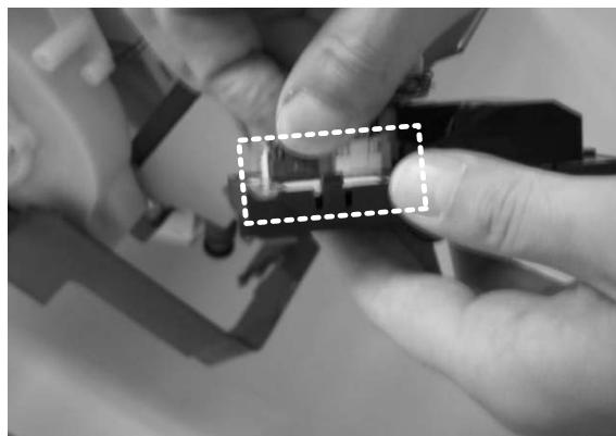
31)The sub.printed board cover is removed. (Hook two places)
