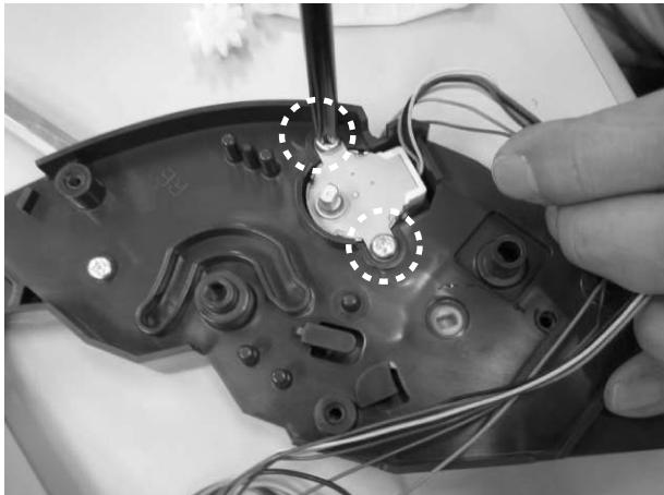
24)The mechanism case is removed. (Hook one place)
