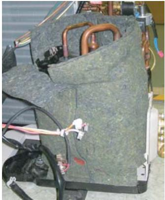
17)A thermistor is removed. (1 place)
