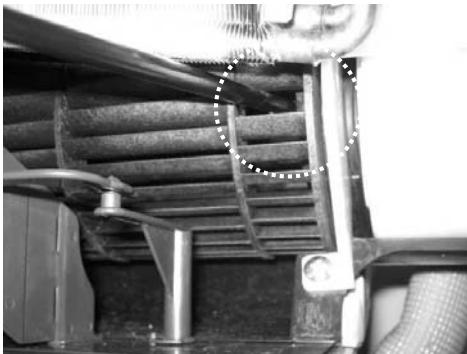
64)The two screws for the fan motor cover fixation are removed.
