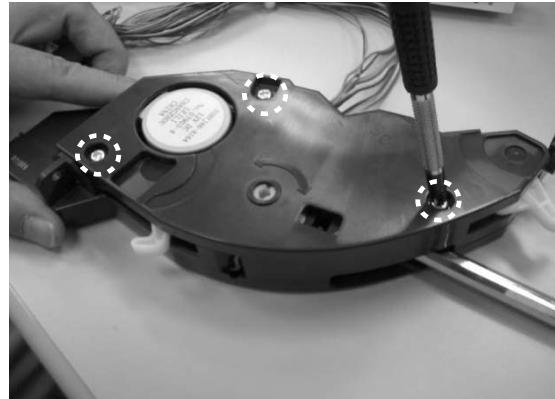
21)The screw that is the fixation of the panel motor is removed, and is turned to the left and it is removed.
