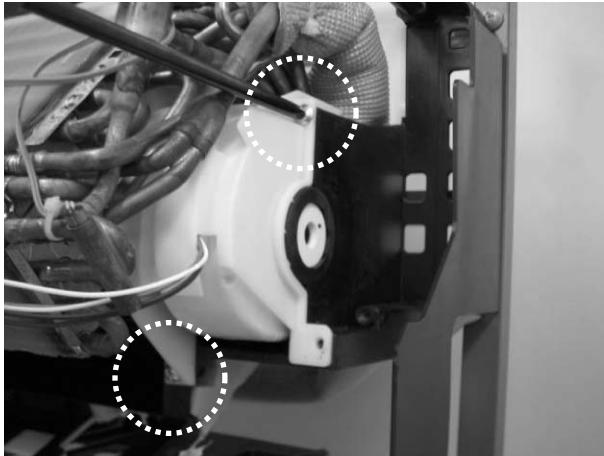
65)The cross flow fan is pulled out at the left of the unit and it removes.
