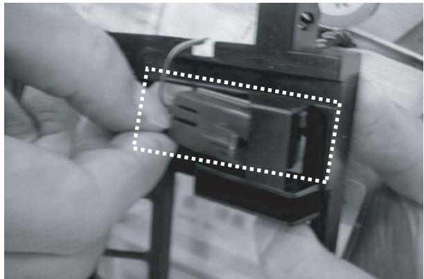
46)The limit switch is removed. (Hook one place)
