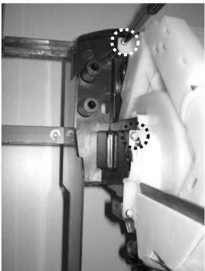
57)Two screws for the evaporator fixation (right side) are removed.
