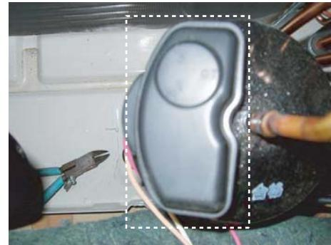
15)A lead wire, a thermistor, and a cover gasket are removed.
