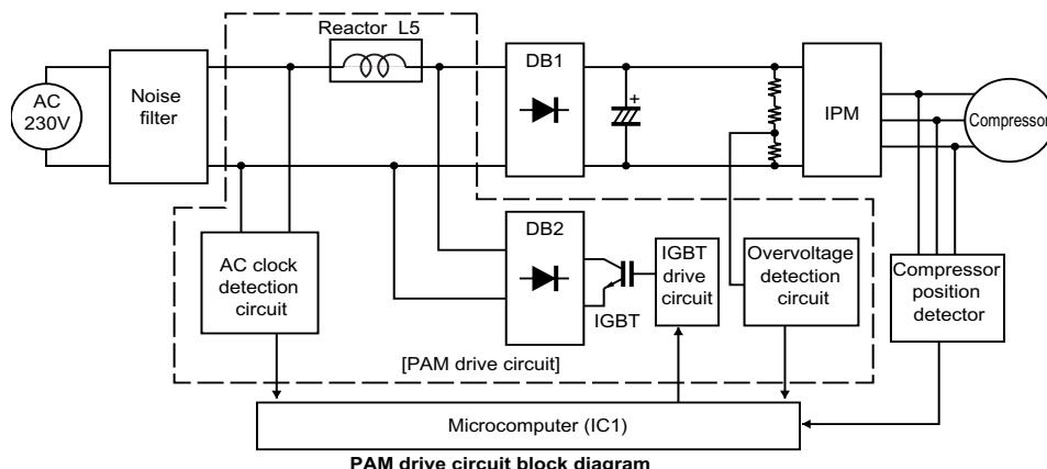
When the IGBT is ON, an electric current flows to the IGBT via the reactor (L5) and diode bridge (DB2).
