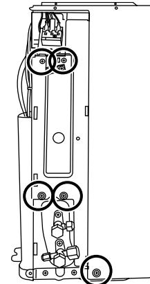
8) The 2 screws on the right-hand side of side cover L is removed.
