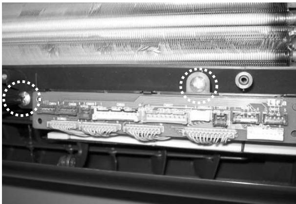
50)P.W.B. assmbly is removed. (2 screws)
