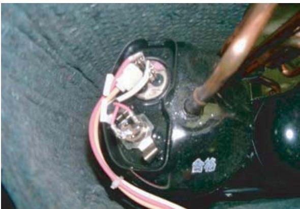
16)The compressor cover is removed.
