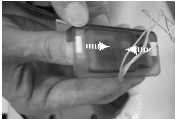
28)The fixing band of the sub.printed boad assembly is cut.
