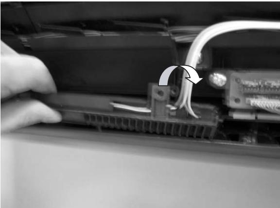
41)Two hooks of the plasmacluster cover are removed by using (-) screwdriver.
