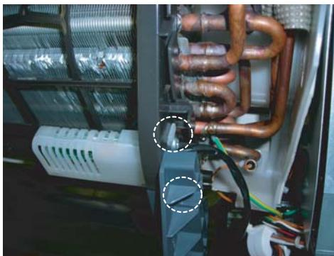
49)The relay printed bord holder removed. (2 screws)
