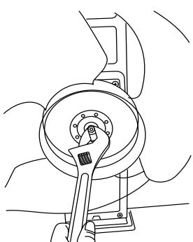
19)The fixed 2 screws of a motor angle is removed.
