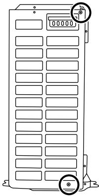
9) The 7 screws of the side cover L and side cover R back is removed.
