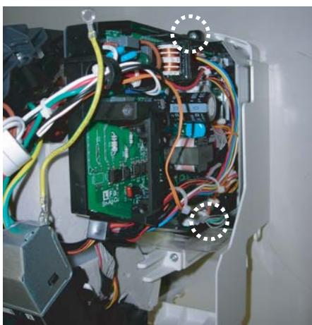
51)The earth cable is removed. (1 earth screw )
