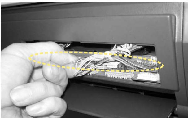
9) The hook three places of the part interior of front panel on are removed.
