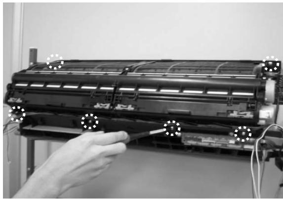
44)Air filter cleaning mechanism assembly is pulled forward and removed.
