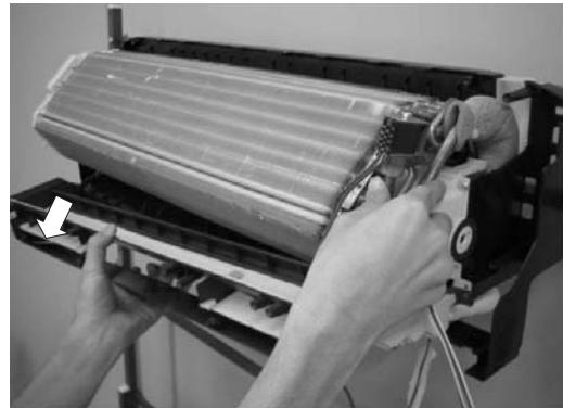
60)Four fixed screws of the vertical direction louver stand assembly removed.
