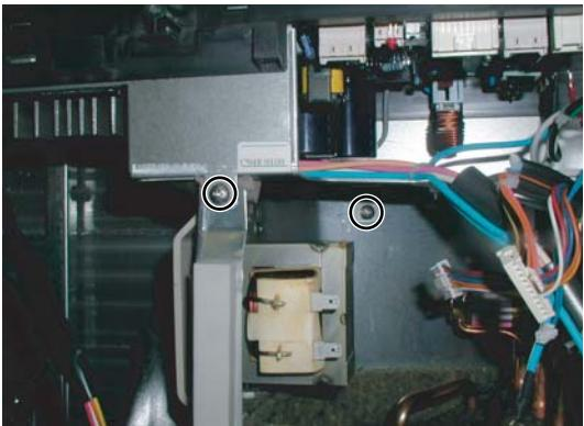
12)A bulkhead plate fixed 2 screws is removed.
