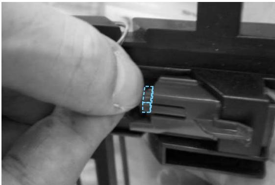
48)The thermally sensitive resistor holder is removed.
