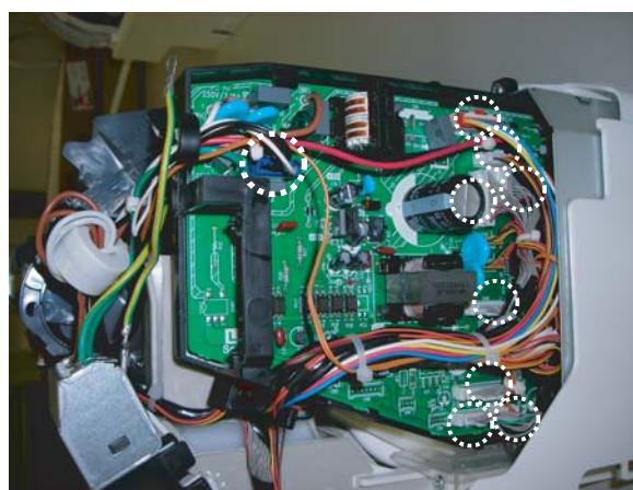
38)The Terminal board removed. (1 screw )
