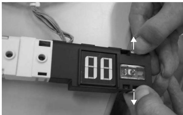
19)The display printed boad is removed. (Hook three places)
