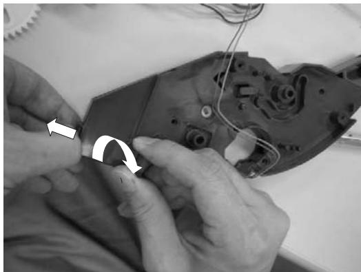
25)The limit switch is removed.
