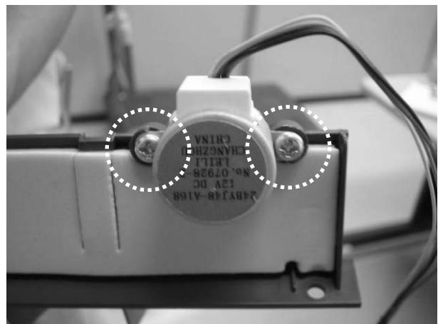
62)The bearing holder is removed. (1 screw)
