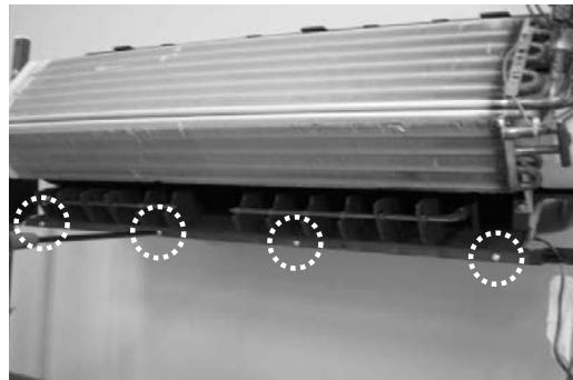
61)Driving motor of the vertical direction louver stand assembly is removed. (2 screws)
