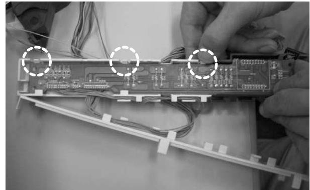
20)The panel mechanism cover is removed. (3 screws)
