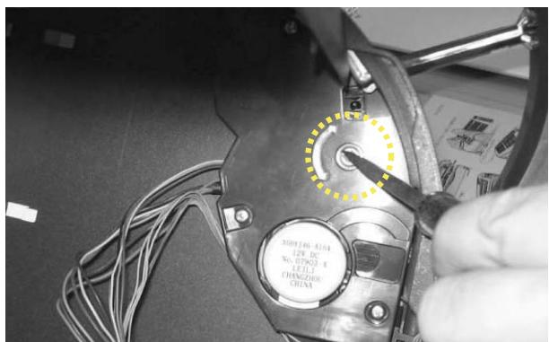
14)The pin that is the fixation of the panel base and the link is removed.
