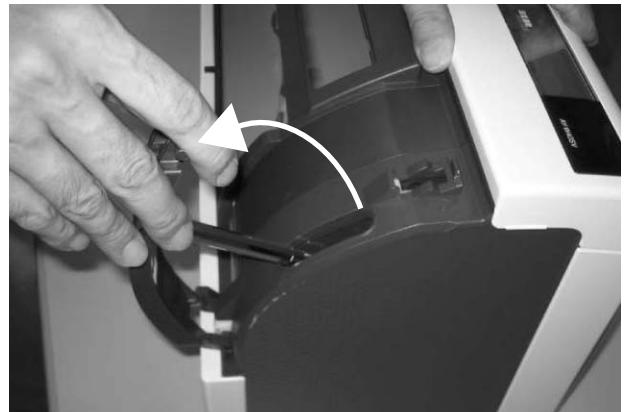
13)The gear is turned, and the panel base is removed. For a minus screw driver etc.
