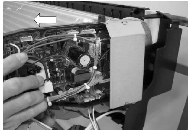
53)The Terminal cover of the Terminal stand assembly is removed.
