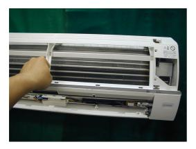
11)Remove a screw fixing the control box cover, and remove it.
