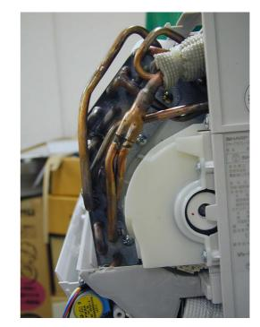
31)Remove the screw fixing the evaporator.
