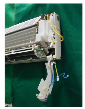
25)Remove a screw fixing the drain pan ass'y and disconnect the motor connector.
