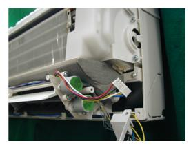
26)Remove 2 screws fixing the holder.
