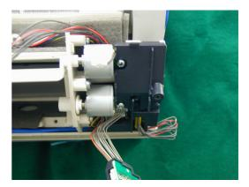
20)Disconnect the connector of Display board.
