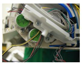
23)Remove a screw fixing the holder.
