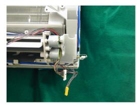
22)Remove the 2 screws fixing the display base.
