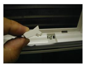
9) Remove 5 screws fixing the front panel.
