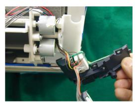
21)Disconnect the connector of Display board.
