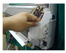
30)Remove the screw fixing the evaporator.
