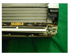
16)Pushing the 2 hooks of the holder, remove the display board.
