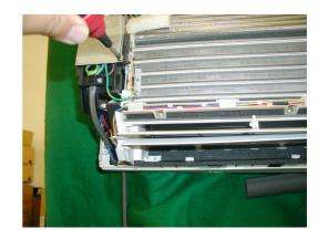
12)Remove the 2 screws fixing the control box.
