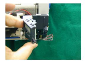
19)Remove the 2 screws fixing the display guide.
