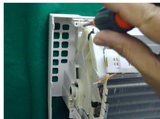
29)Remove the drain guide.
