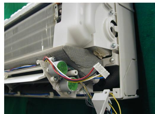
26)Remove 2 screws fixing the holder.
